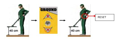
**8.** If the ground setting cannot be done as a result of the actions explained above, the "SENSITIVITY" level of the device should be reduced and the actions explained above should be repeated.
